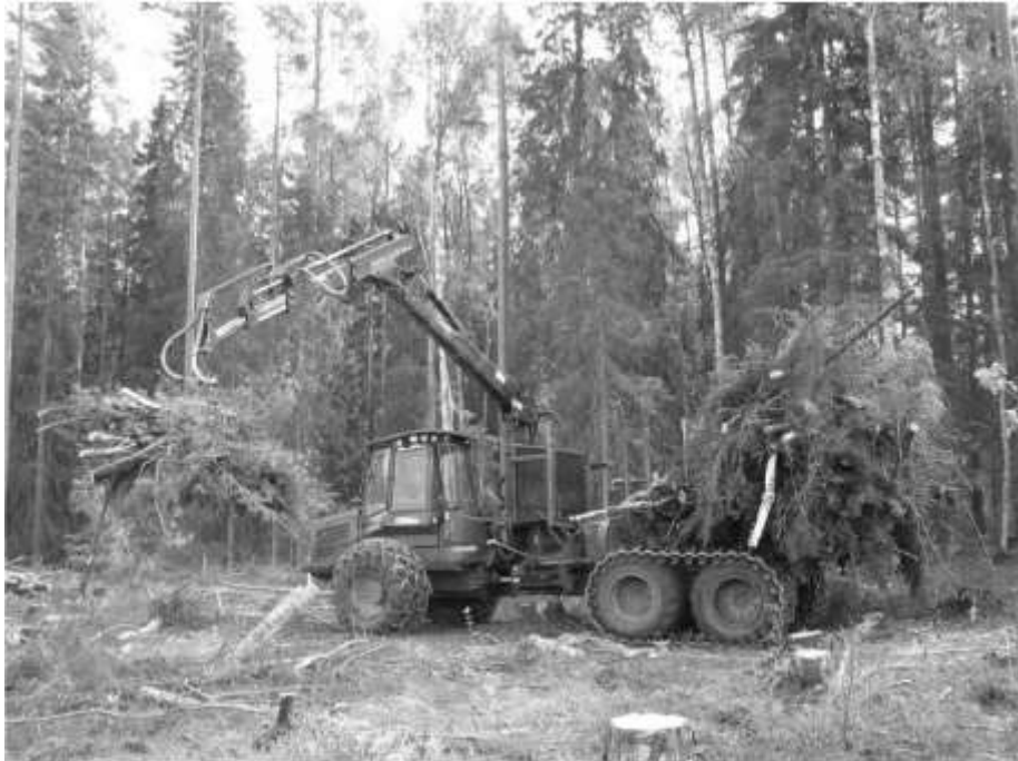
Figure 3. Loading LR onto a forwarder commencing at the rear (Laitila et al. 2013).
