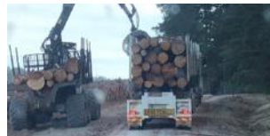
Figure 6: The loader using the uprights to determine load height.
