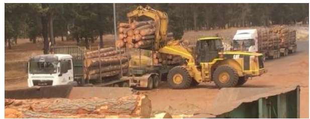
Figure 11: The first bay to be unloaded is the centre bay. It is placed on the ground next to the in-feeder.
