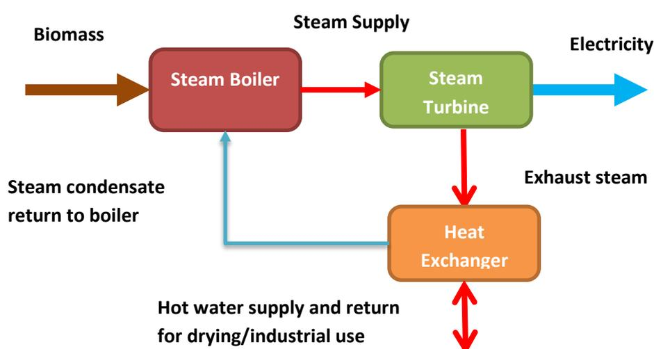
Figure 4: Basic flow diagram for Steam based Rankine cycle
