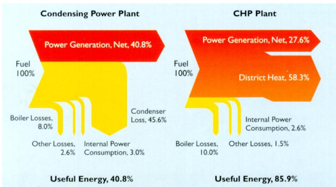
Figure 1: Comparison a traditional thermal power station and Combined Heat and Power (CHP)<sup>1</sup>
