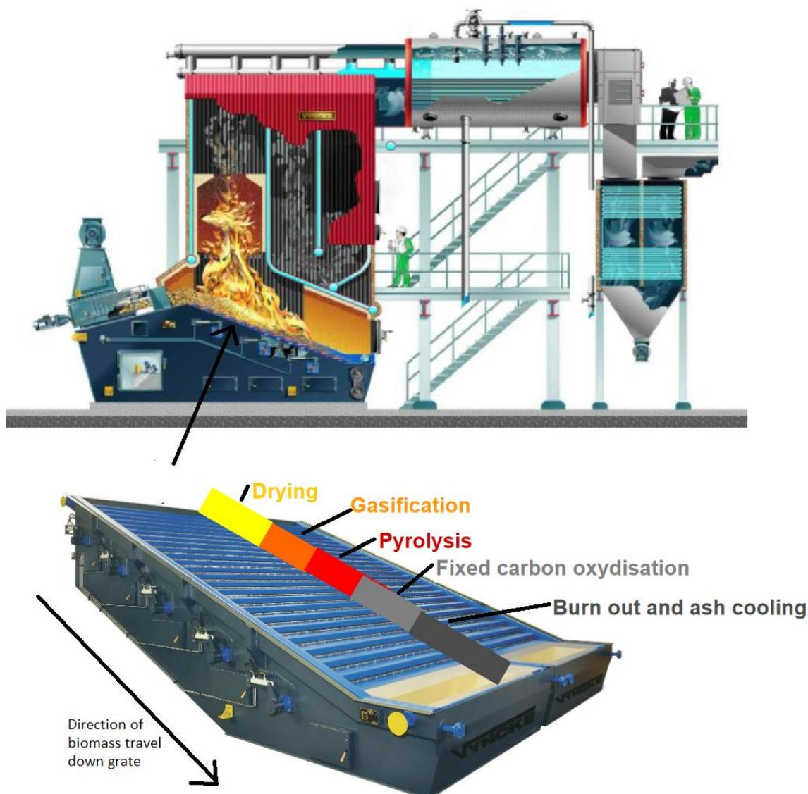
**Figure 5: Overall schematic of boiler and detail shown of moving stepped grate (courtesy of Vyncke<sup>8</sup>)**
