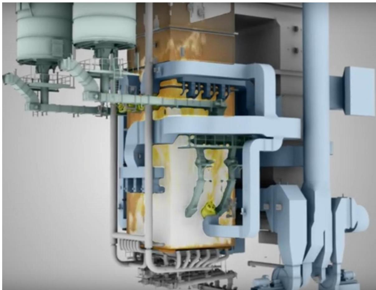
**Figure 6: Valmet Bubbling Fluidised Bed boiler**
